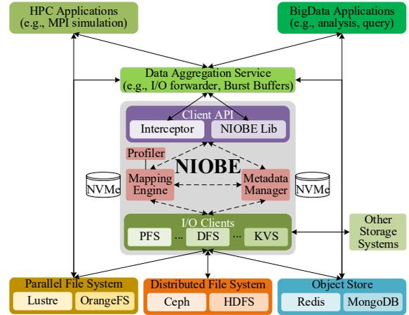
Fig. 1: Architecture design of NIOBE
